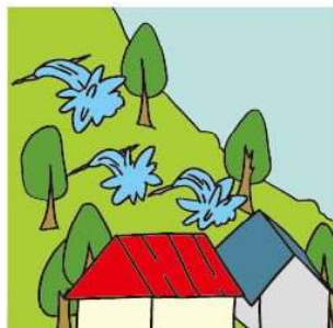
Water spurts from the slope.
